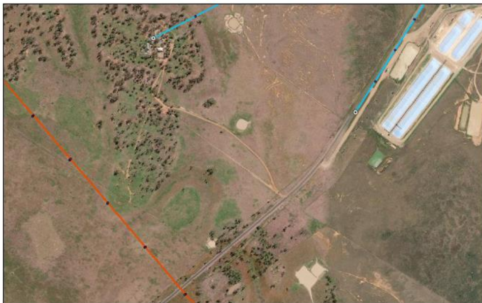
Figure 2-2: Existing 22 kV (blue) and 132 kV (orange) transmission lines
